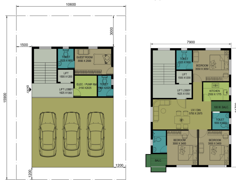
Typical Floor plan for 1st, 2nd and 3rd floors
